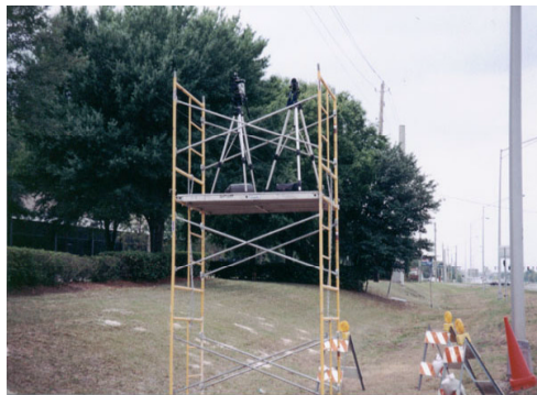
Fig. 3 – Field setting-up of video cameras
