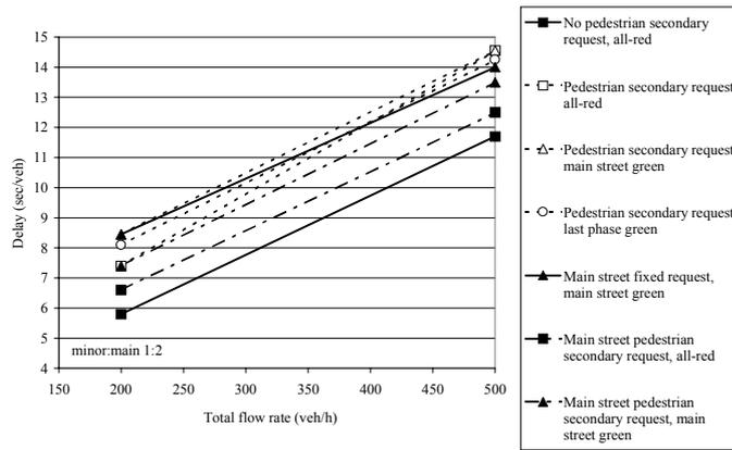
Fig. 2 – Results of three-phase control with pedestrian crossing
